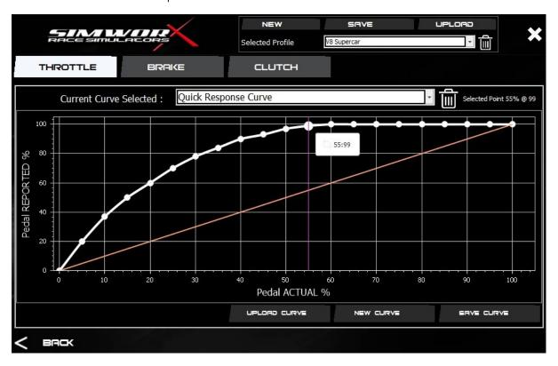
Once the curve is as required save the curve using the "SAVE CURVE" button. You will then be prompted to name the curve, ensure you give the curve a unique name to prevent saving over other curves.
