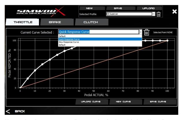
\*\*NOTE: when changing a curve, it will appear as the white line, while the red line will indicate the curve currently loaded on the pedal set.
