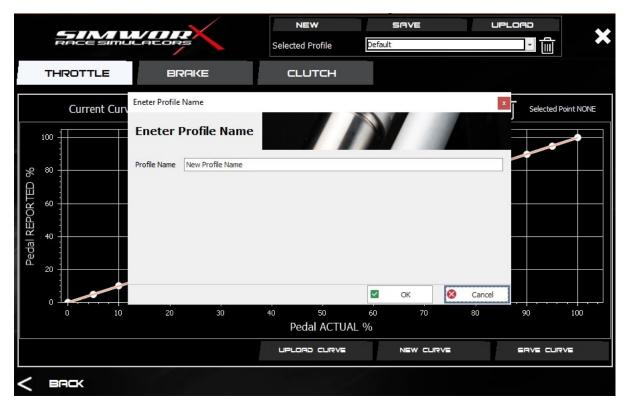
Enter your desired name for the new profile and hit "OK". This will create the new profile and give each pedal a default linear curve.
