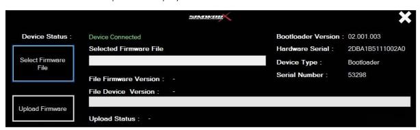
Press the "Select Firmware File" button and navigate to the save location of the firmware file, select the file to load.
