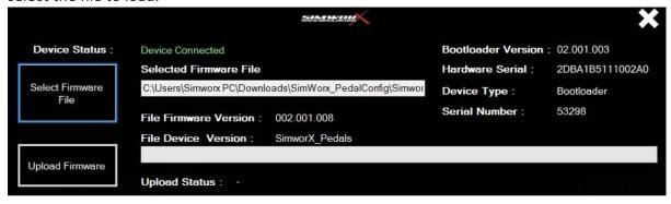
Press the "Upload Firmware" button to begin to upload.
