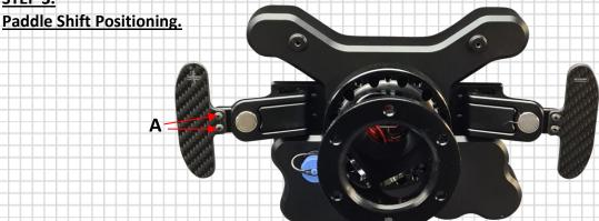
The Carbon Fibre Shift Paddles can be adjusted in or out by 10mm each side to your preferred position. Loosen the two cap screws (A) slightly and slide in or out to your preferred position. Depending on the wheel that is fitted, the paddles themselves can be spaced further out by using the supplied spacer and screw pack to space it out to your preferred position.
