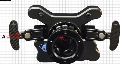
The Carbon Fibre Shift Paddles can be adjusted in or out by 10mm each side to your preferred position. Loosen the two cap screws (A) slightly and slide in or out to your preferred position. Depending on the wheel that is fitted, the paddles themselves can be spaced further out by using the supplied spacer and screw pack to space it out to your preferred position.
