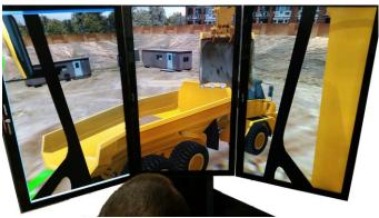
An accurate representation of a typical machine cab layout using replica controls, operators chair, built in PC, sound system, vibration transducers and dedicated software. Features typical Joysticks and track pedals with handles, safety handle and comes in single or optional triple screen formats.
